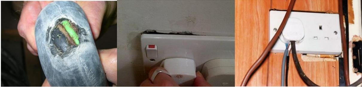
Examples of unsafe electrical plugs, sockets and leads
