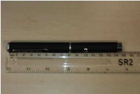
The laser pointer is matt black with a silver control button, clip, top and edge of laser aperture. It is approximately 15 cm long and 1 cm diameter.
