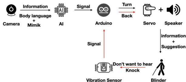
Figure 3. **Prototype Function**
