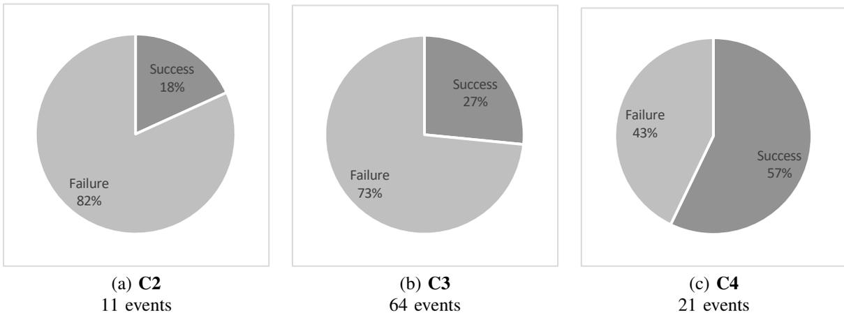
Fig. 3. Interaction success rates by condition. (a) C2, haptic only, (b) C3, haptic and visual only, (c) C4, haptic, audio and visual cues. The legends also shows the number of interaction events per condition.
