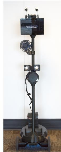
Fig. 2. The tele-operated Omni Robot was instrumented with a fan, mounted just below the screen, speakers, a screen, as well as a visible set of eyes.
