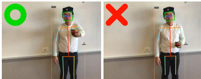
Fig. 1: We detect whether a user is initiating a handover from a single RGB image. Handover gesture is correctly detected (left column). No handover activity is detected (right column).
