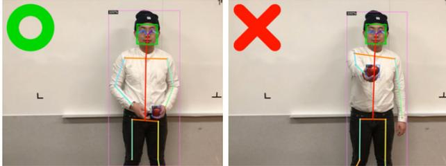
Fig. 5: Some failure cases. False positive (Left). False negative (Right)
