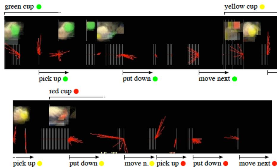
(a) Object and motion chunks created through task demonstration
